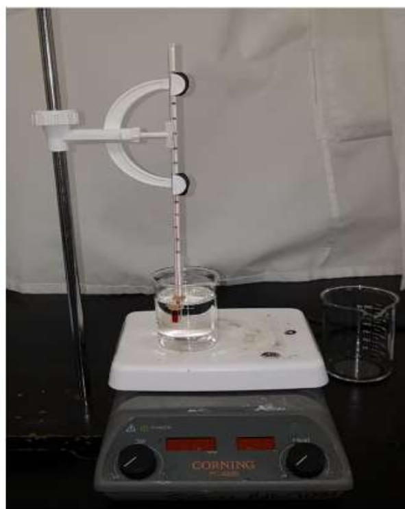
Fig1: Set up of the apparatus for melting point experiment
